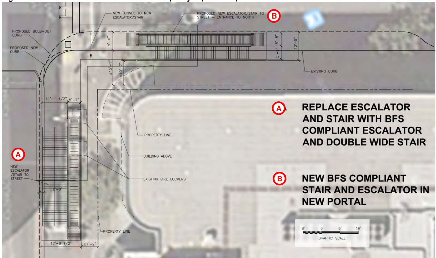
Figure 25: North End of Concourse to Surface Capacity Expansion Options
